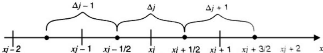
cell end points:  $0 = x_0 < x_{j-\frac{1}{2}} < x_N = 1 \quad j = 1, 2, \dots, N$
