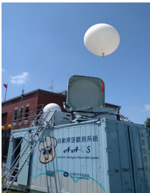
圖 3.3.2 TAHOPE 實驗期間 AAOS 於新竹氣象站自動施放之探空氣球。 Figure 3.3.2 Weather balloon autolaunched in Hsinchu weather station during TAHOPE
